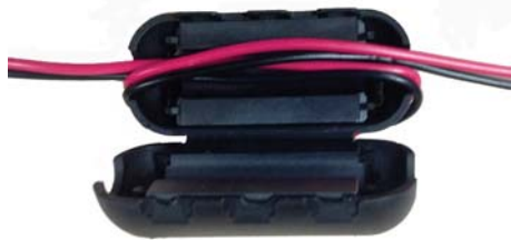
Figure 6. Ferrite Clamp Installation
